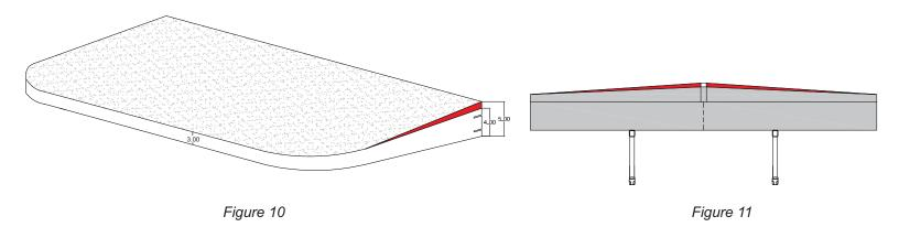
Specifically to fix the problem <u>foam warping as the panel ages</u>... you have to remove the foam panel from the skin, rotate it and reinsert it into it. Doing this, the warped side will remain on the bottom and top will have a brand new good surface for the water to run off.
