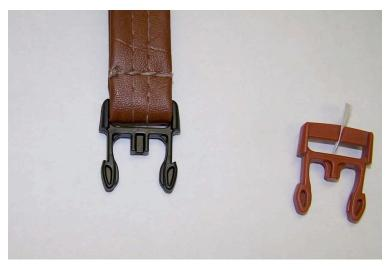
On the left hand side of this picture above is how the clip looks attached to the vinyl spa cover strap. On the right hand side of this picture above is a clip that has been modified to use to repair a broken clip. The top crossbar has been cut.
